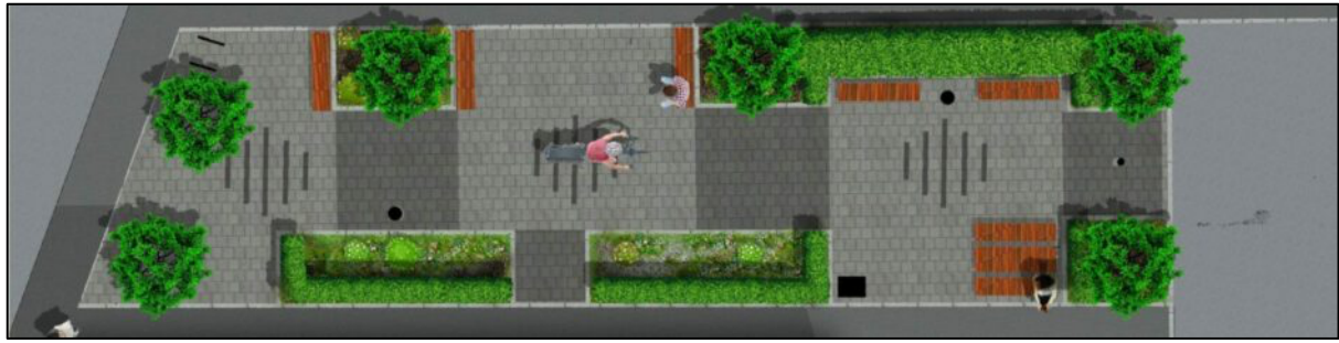
Figure 10: Retrofitting rain gardens into projects to retard flow of water into sewers. (Image Sustrans).
