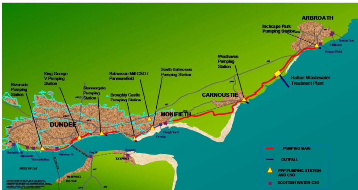
Figure 1: Pumping station network and outfalls in the TEF region (Carr, 2004, from University of Abertay report, 2011).
